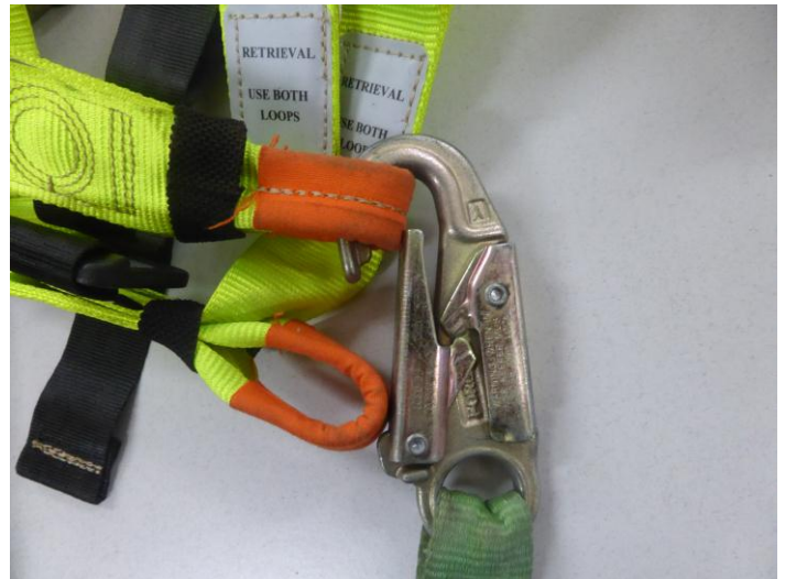
Figure 1; Insert one loop at a time – pulling the loop all the way through.
