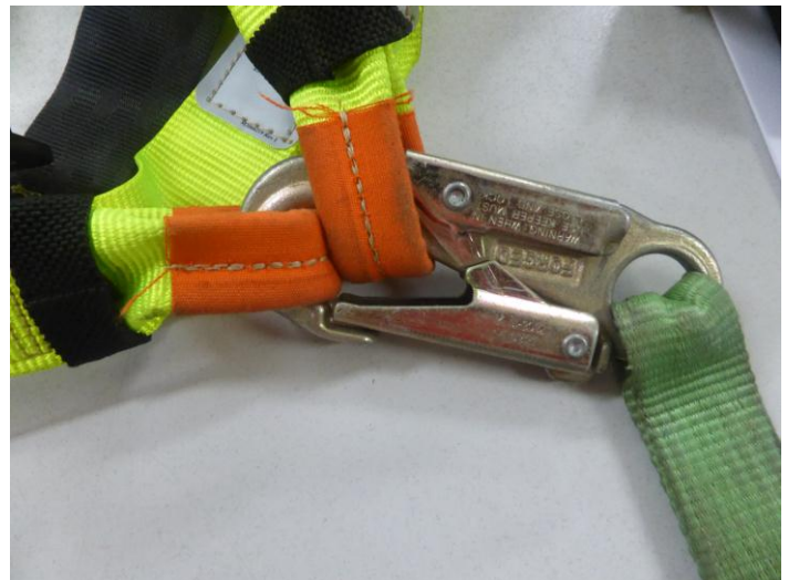
Figure 2. Once the first loop is on, feed the second loop through and close the hook.
